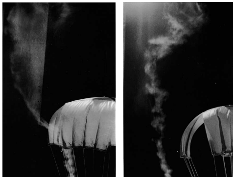
(b) 烟雾示踪显示流场 [9] ( A=3, \alpha=0^\circ, Re=3.9 \times 10^5 )
