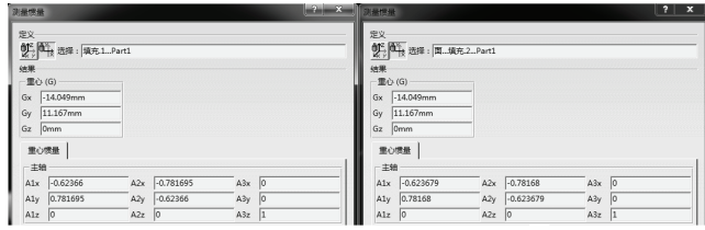
(a) 样条叶片截面前缘的重心及主轴 (b) 圆弧前缘叶片截面的重心及主轴
